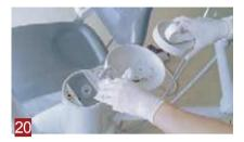
20.Remove the drainage rod, open the drainage cover, and check if wiping is needed. If so, wipe it clean with a cloth dampened with disinfectant before reinstalling.
