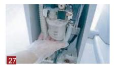
27. Lift the waste collection tank upward to check whether the trigger switch is normal.
