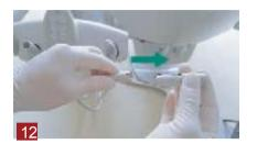
12 : Use 1L of 500mg/L chlorine containing disinfectant each for strong and weak suction to flush the saliva suction tubes and drainpipes. Pour 500ml of disinfectant into the spittoon to disinfect it. The pull out the heads of the strong and weak suction tubes.
