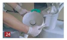
24.Reinstall the spittoon by turning it clockwise.
